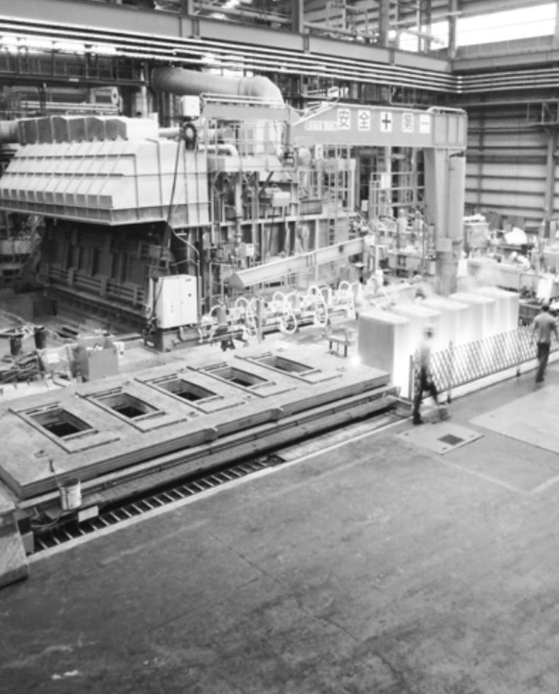
The scrap is then pushed into the molten metal bath at the rear of the chamber where it is melted in a constant stream of hot metal flow recirculating from the main clean aluminium chamber. Heating is provided by gas fired twin head regenerative burners.
